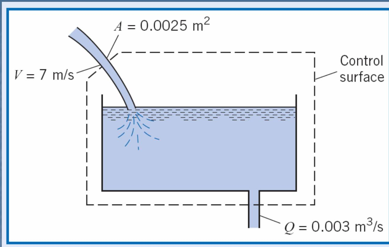
Find the rate of water accumulating in or evacuating from the tank?
