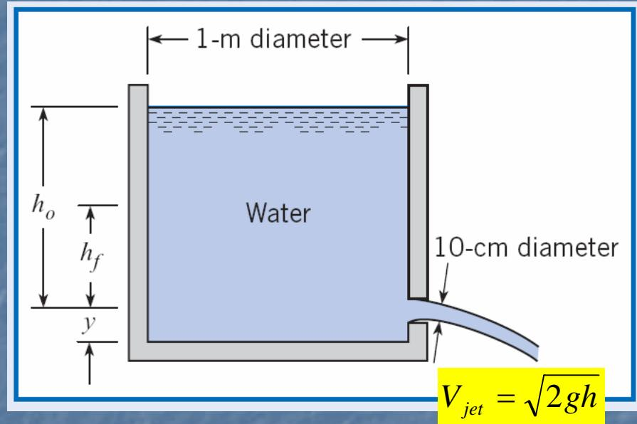
How long will take ( $t=?$ ) for the water to drop from  $h_0= 2m$  to  $h_f=0.5m$  ?
